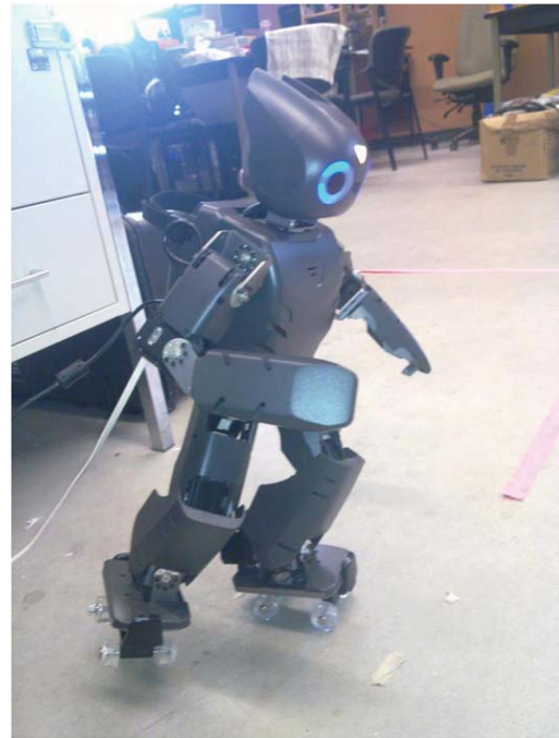
Fig. 15. The robot using a statically stable gait on roller skates.
