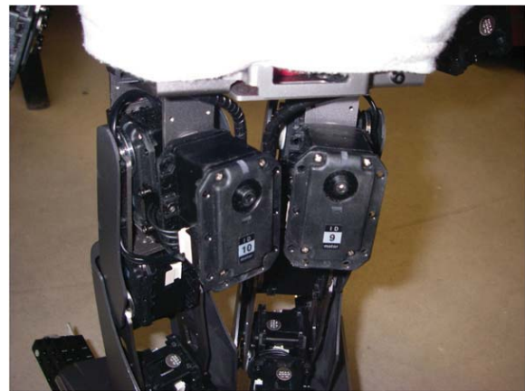
Fig. 17. The motors in the robot's hips can collide if the legs are turned outwards too far.
