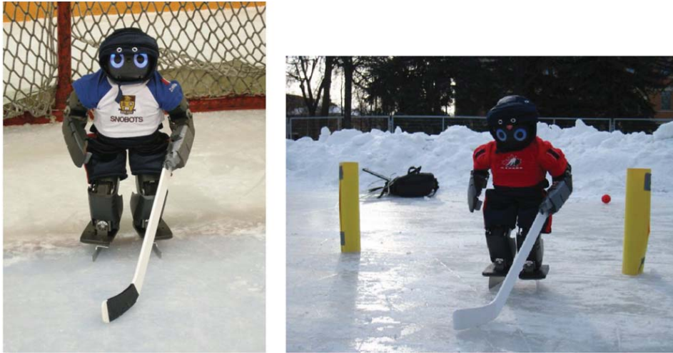
Fig. 10. Jennifer, the robot used in our experiments, skating on an indoor (left) and outdoor (right) ice surface. The hockey stick was used to interact with a foam ball and did not serve as a balance aid. The helmet, shirt and trousers helped protect the motors from cold and moisture.
