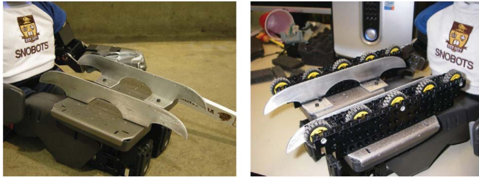
Fig. 12. The robot's ice skates (left) and inline skates.
