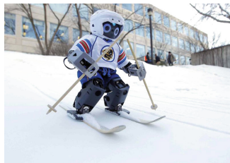
Fig. 6. A humanoid robot equipped with skis demonstrating alpine skiing. We use the “do the shake” policy to control the robot’s pitch and roll while skiing. (Winnipeg Free Press [16])
