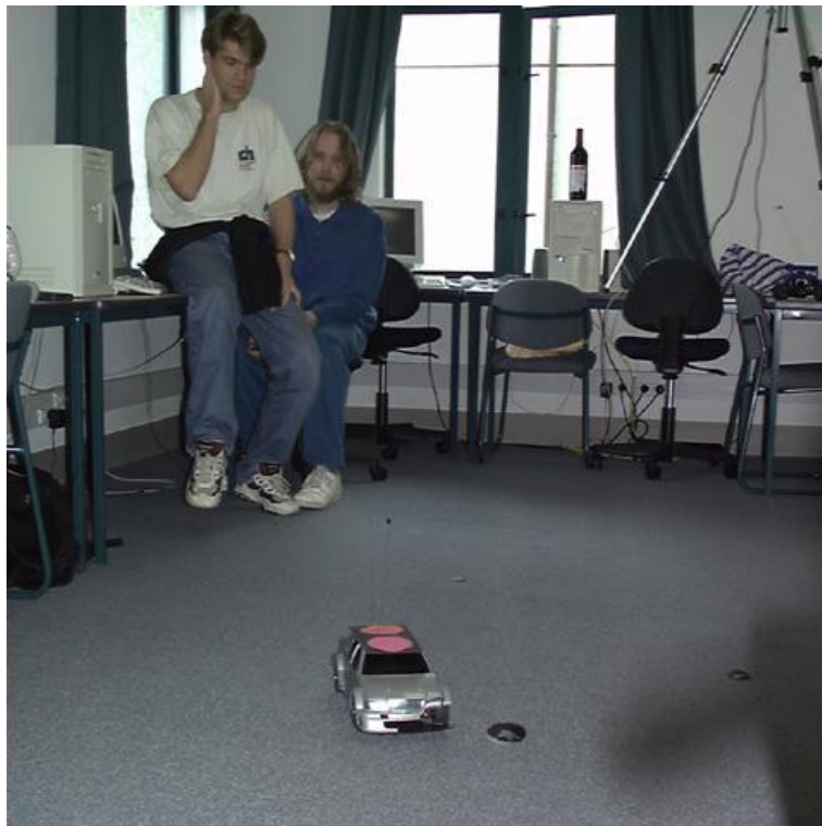
Figure 1: Aucklandianapolis at the University of Auckland. The tripod of the vision system can be seen on the top right corner of the image. The video camera is just out of the picture. The video server determines position and orientation of the cars by bright dots on the car. As can be seen, the speed trials took their toll on our cars.
