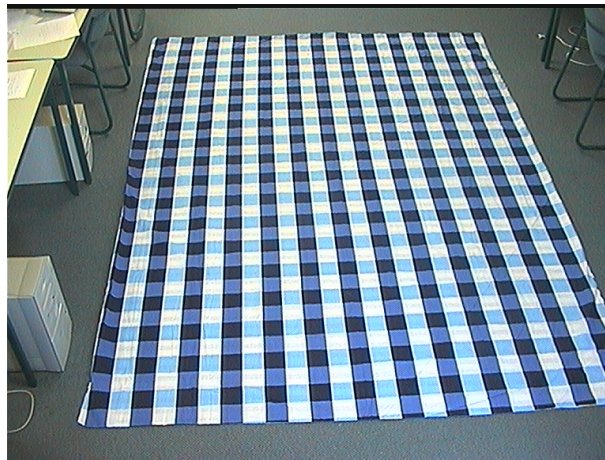
Figure 2: Calibration Pattern as seen by the Camera
