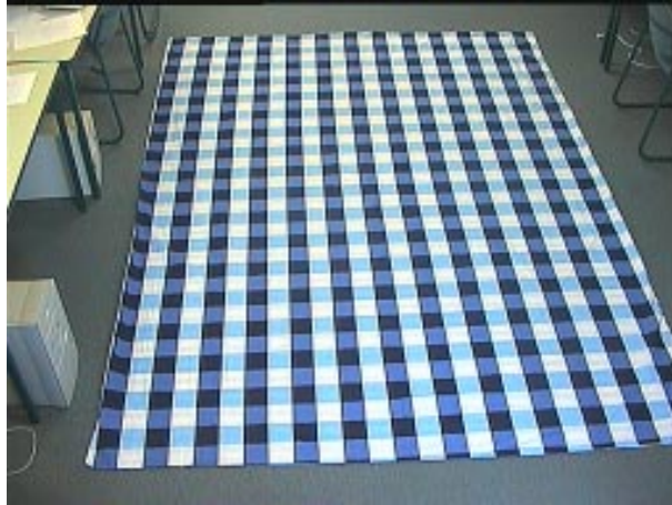
Figure 1: Calibration Pattern as seen by the Camera
