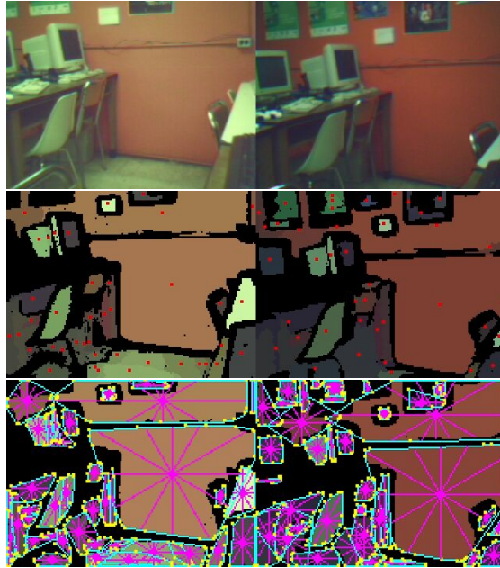
Fig. 1. Segmented regions (middle) from the raw image pair (top) after blurring and edge detection, with convex hulls plotted (bottom).
