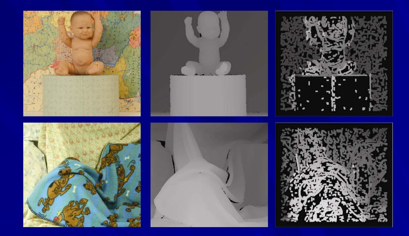
Robustness to camera jitter means knowledge of epipolar lines cannot be assumed, nor rectified stereo frames. Cheap equipment also renders color calibration unreliable. The result is a more robustly-applicable approach to stereo vision because of a lack of reliance on these traditional assumptions
