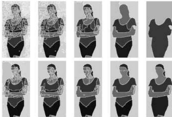
Figure 9: Results of scale-space watershed segmentation using Gaussian diffusion (Top) and CLMC (Bottom) to reduce over-segmentation. Images from (Vanhamel et al., 2003).
