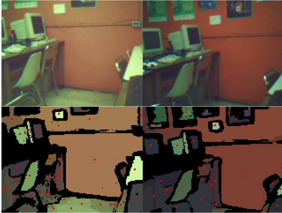
Figure 10: The region segmentation (bottom) is produced from the raw image (top). The dot inside the regions represent the centroid point. Images from (McKinnon et al., 2005).
