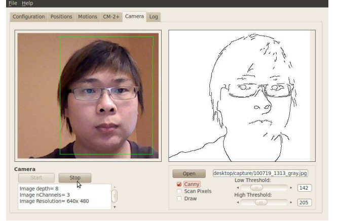
Fig. 9. OpenCV image processing module
