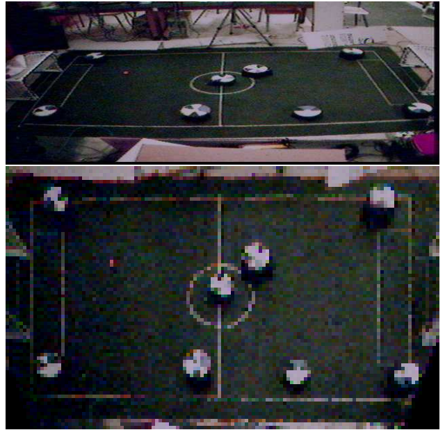
Figure 1: Captured field and corresponding low-resolution interpolated image
