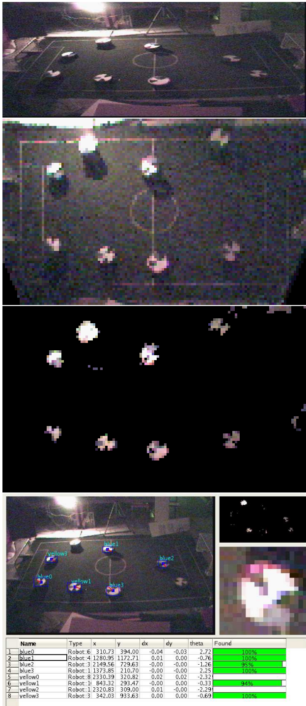
Figure 4: A situation with very poor lighting conditions (top), the interpolated and motion-detected images (middle) and Ergo output (bottom)
