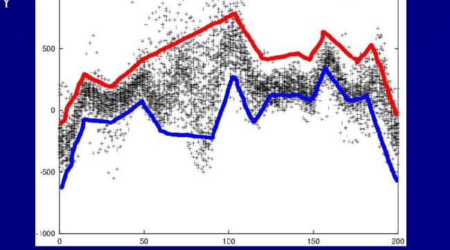
Most readings fall in a small band. Analyzing this walk produced upper (red) and lower (blue) threshold limits to be used in a threshold controller
