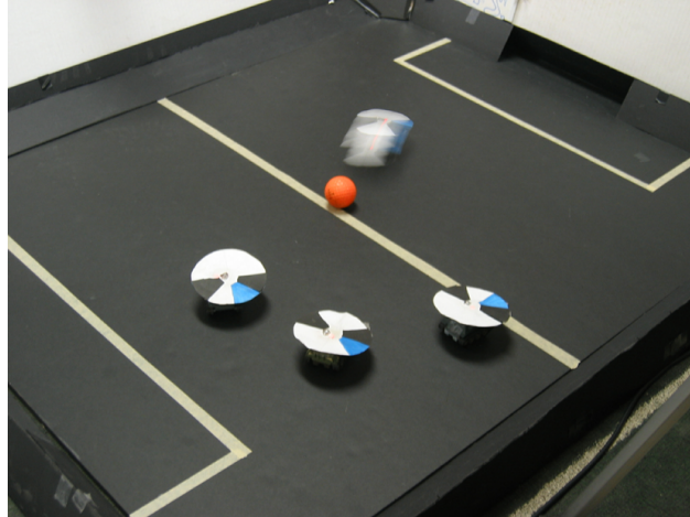
Figure 8: Soccer competition using 2" IR controlled tanks on a tabletop field.
