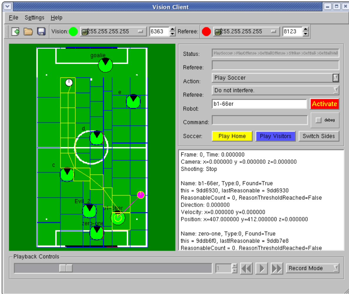
Figure 5: Path planning using Flexible Binary Space Partitioning
