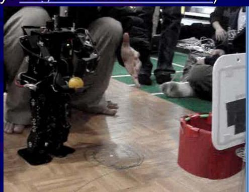
Weightlifting: lift as many CDs as possible on a bar: walk 30cm with the weight below the head, 30cm with the weight above – drastically but predictably changing COM
