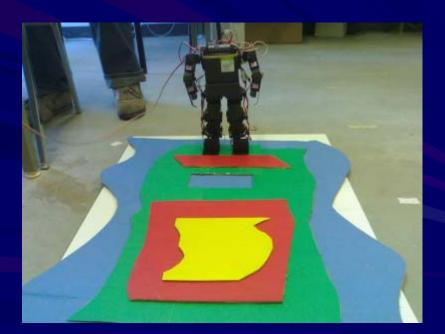
Obstacle Run: Move through a 3m long region without touching any of 3 types of obstacles: walls, holes, gates. Gates can be crawled through (complex motion planning)
