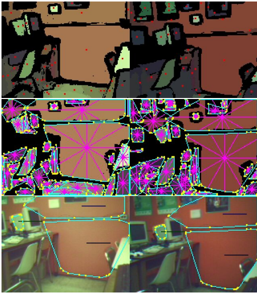
Figure 2: Segmented regions (top), convex hulls and signature lines plotted (middle), matched regions (bottom).
