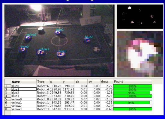
Maintains a frame rate of 28-35 fps while tracking eight robots.
