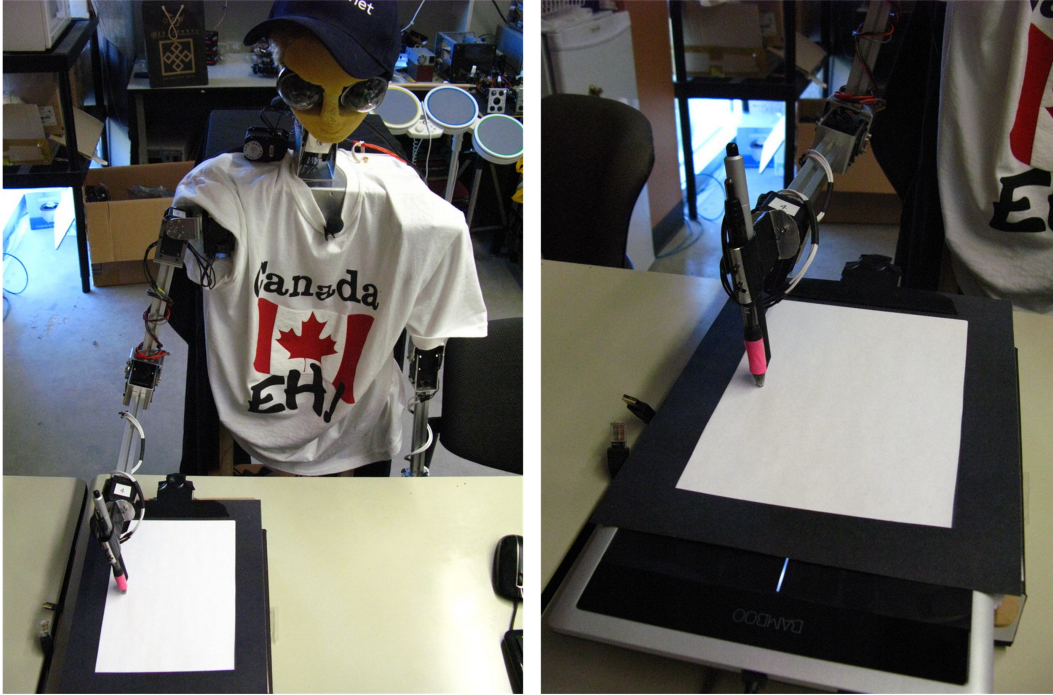
Figure 4.7: Experimental setup using a Wacom Bamboo tablet (CTH640M), Betty, camera and pen.
