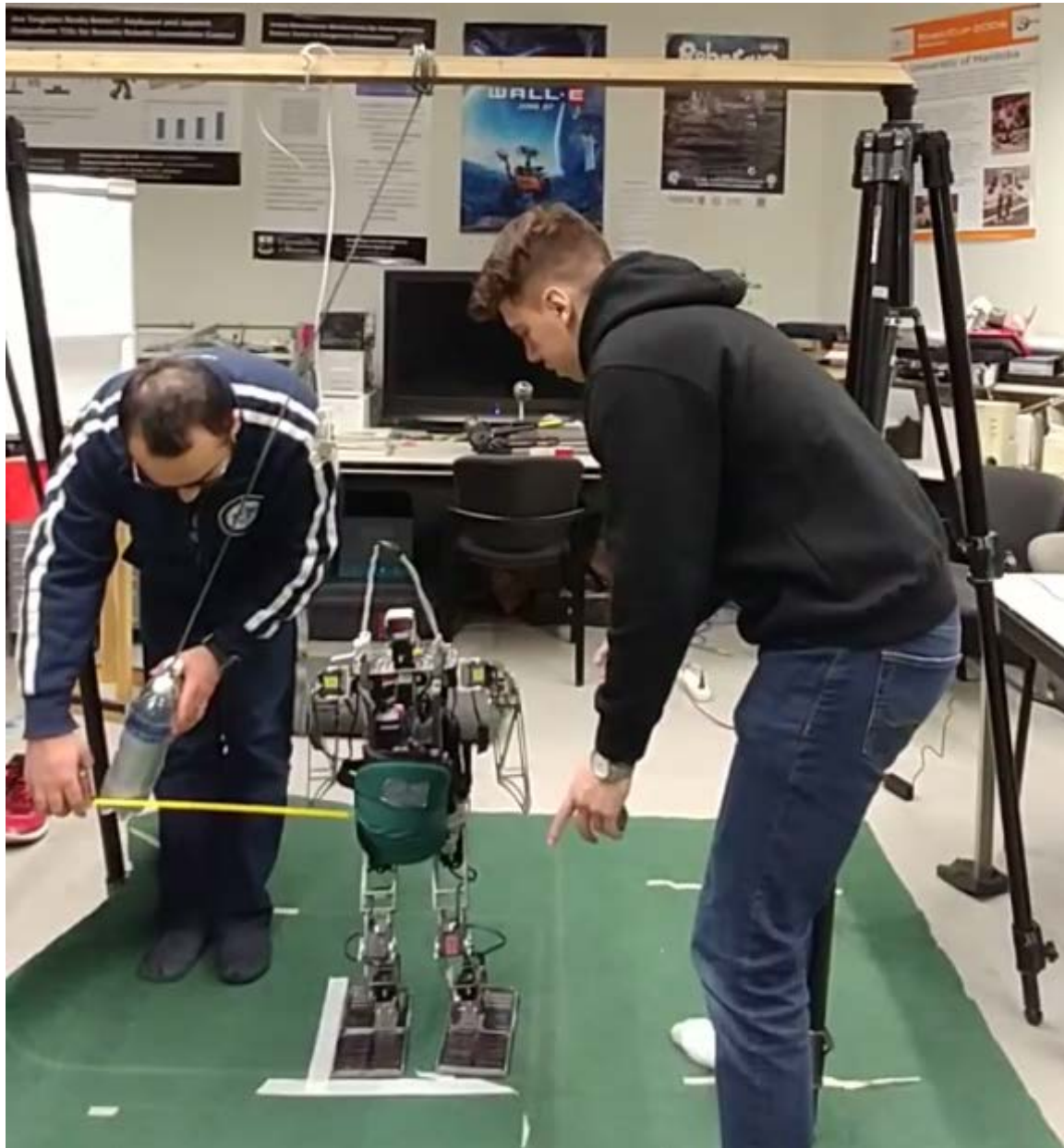
Figure 4.5: Experimental setup in the real world on the carpet surface for both RL and DRL.
