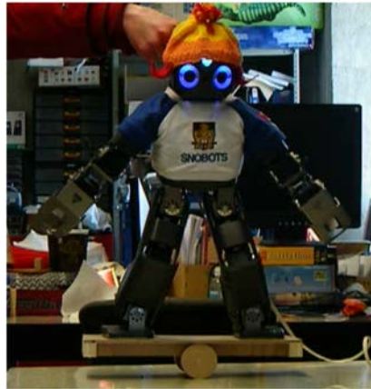
Figure 2.4: DARwin-OP humanoid robot, on a Bongo Board [Baltes et al., 2014].
